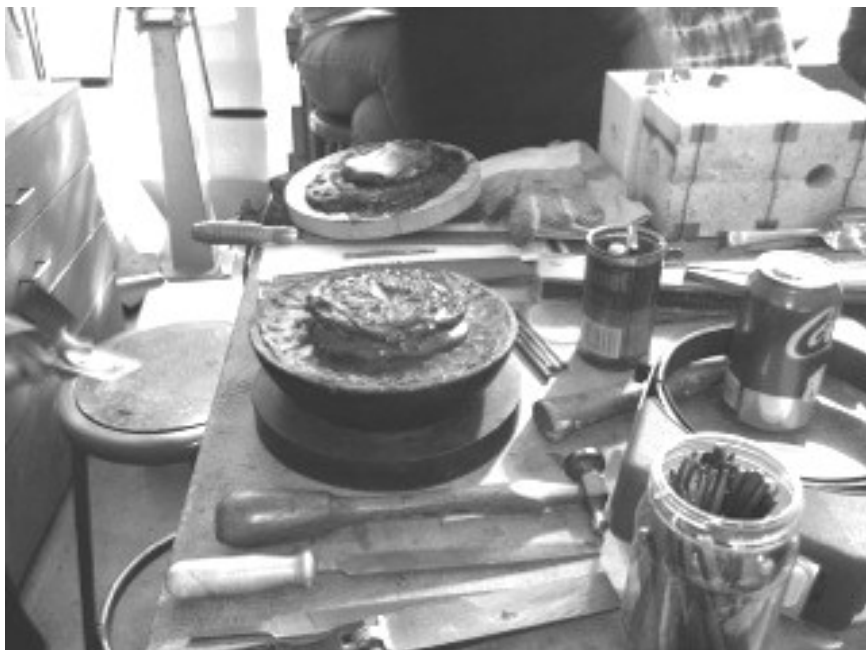
Pitch bowl, chasing hammer, file, and hand-made punches. The tools of the Chasing and Repoussé trade
